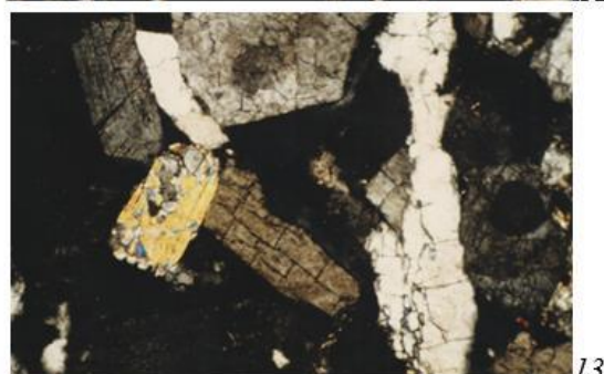
Fig. 12-13: Observation of thin blade of the beige vosgian sandstone before (12) and after (13) treatment with pH 12.6
